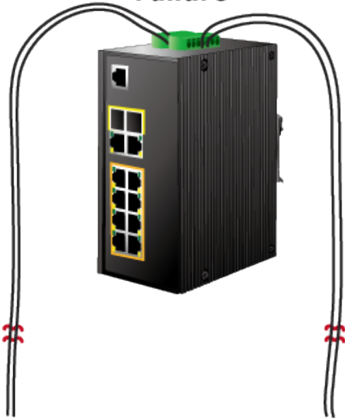
DC/DC Power Failure
